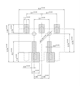
Note: 1. The above figure is the figure viewed from the connector mounting side . 2. Tolerances are non-cumulative: ±0.05 mm for all centers. The dimensions above should serve as a guideline. Contact JST for details.
