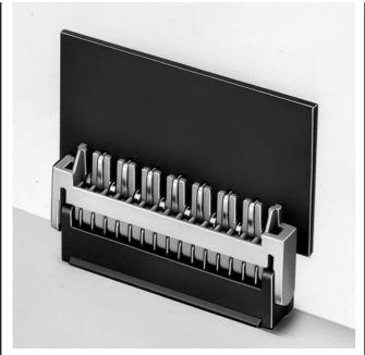
Hinge type board to board connectors which allow mated PCB's to move 90° in respect to one another while electricity is turned on. The hinge compensates for slight misalignments between circuit boards to assure a secure connection even if the boards are laterally out of line.
