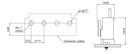
Note: 1. The figure of PC board layout is the figure viewed from the connector mounting side.
