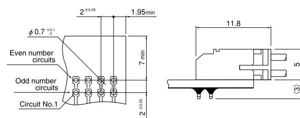
Note: 1. The above figure is the figure viewed from soldering side.
