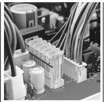
This 3.96mm pitch insulation displacement connector is used with printed circuit boards. Since the connector can accommodate 18 AWG wires and has a large pitch, it is ideal for connecting power supply circuits.
