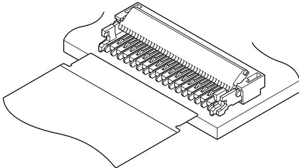
**0.2mm pitch FVXS connector for FPC has been developed for small portable equipment for which low profile and miniaturization are required. Positioning of FPC is easily conducted by inserting FPC into connector until its shoulder touches to the transverse U-shape groove. This connector also has the structure that tension due to handling of FPC is absorbed by socket and reinforcing tab.**
