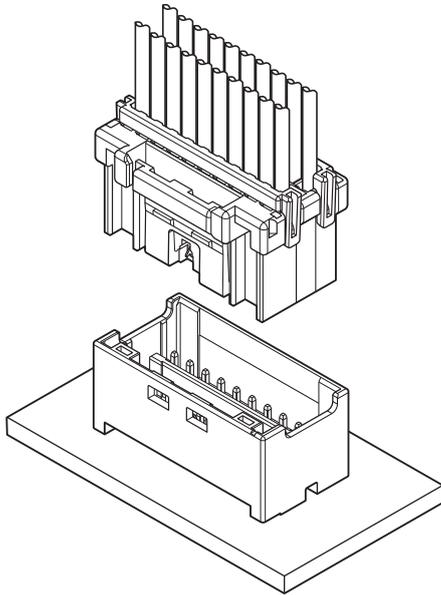
This PID connector is a 2.0 mm pitch box type wire-to-board connector with secure lock device, and it has the mechanism for detecting half mating, which is possible to judge electrically whether its state is the complete or incomplete mating by the circuit of detecting half mating provided at the part of connector.
