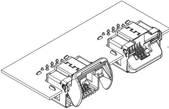
This is an interface connector compatible with RJ45 and designed as low profile and space saving type with a cover opening and closing structure.
